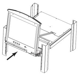
3. Rotate the LCD module all the way down, then pull and let go of the rear catches to release the LCD module
